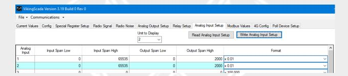
These scaling values are used only in the master and not sent to the slaves. The results of the scaled slave inputs can be seen on the Current Values tab or in Modbus registers 15385 - 16376 (768 - 799 for the master's scaled inputs).
