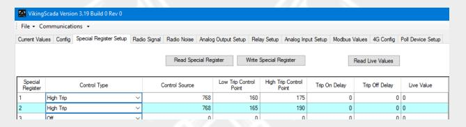
Any relays that are aimed at 883 and 884 will then be driven by these special registers as shown for the first two relays. By setting these parameters the level control can quickly be implemented. The high / low trip points may be changed by any local or remote Modbus device, typically a flat panel display.
